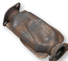
Physical Impact Damage.
