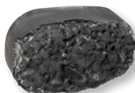
Improper Air/Fuel Ratio or Secondary Ignition System Misfires. Thermal Breakdown Due To Unburned Fuel.
