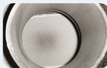
Normal light gray coloration of converter inlet – indicates good mechanical operating condition.
