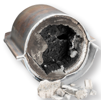
Improper Air/Fuel Ratio or Secondary Ignition System Misfires. Thermal Breakdown Due To Unburned Fuel.
